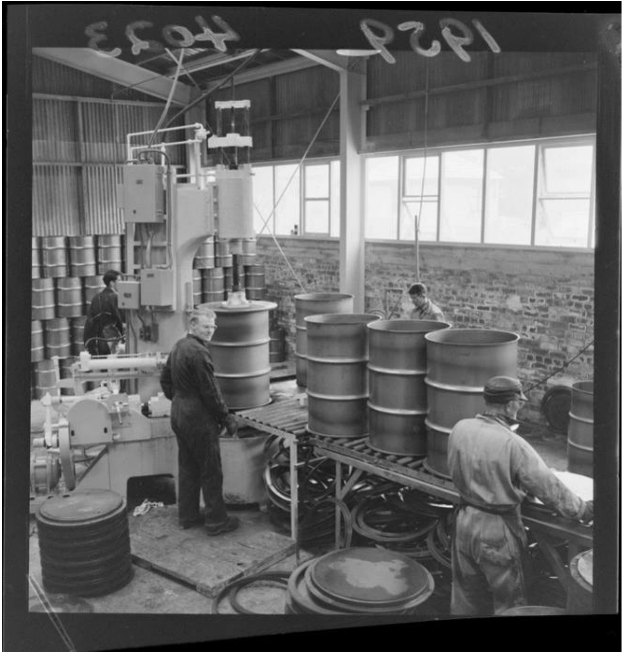
Men making tin drums at a factory, Tawa, Wellington Date 25 Nov 1959 Reference EP/1959/4023-F Part of Evening post (Newspaper. 1865-2002) : Photographic negatives and prints of the Evening Post newspaper / Negatives of the Evening Post newspaper
